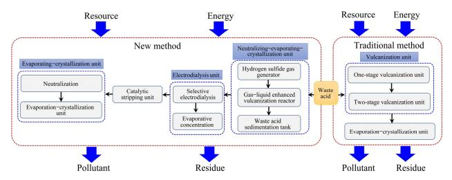
Fig. 1 System boundary of two strategies for waste acid treatment in zinc smelting
