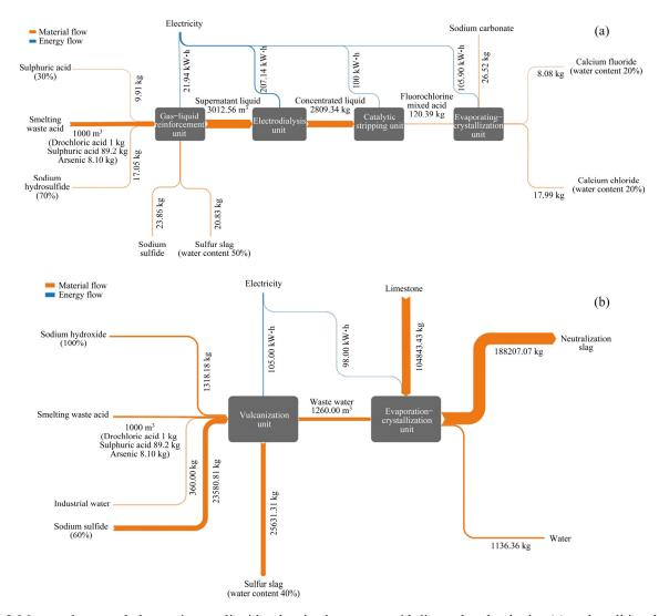
**Fig. 2** Mass and energy balances in gas-liquid vulcanization waste acid disposal technologies (a) and traditional lime neutralization method (b)
