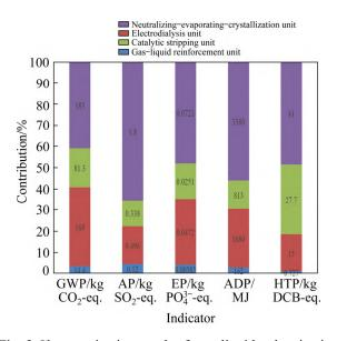
Fig. 3 Characterization result of gas-liquid vulcanization waste acid disposal technologies
