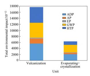
**Fig. 6** Total environmental impacts of traditional lime neutralization method
