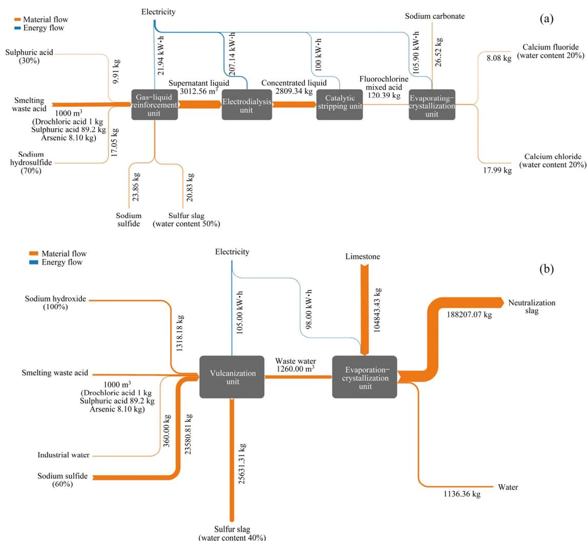
**Fig. 2** Mass and energy balances in gas–liquid vulcanization waste acid disposal technologies (a) and traditional lime neutralization method (b)
