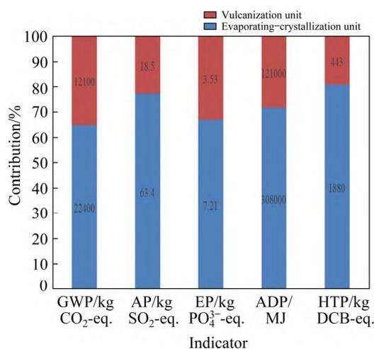
**Fig. 4** Characterization result of traditional lime neutralization method
