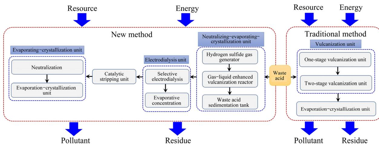
Fig. 1 System boundary of two strategies for waste acid treatment in zinc smelting
