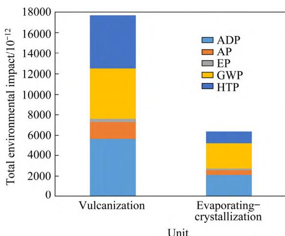
**Fig. 6** Total environmental impacts of traditional lime neutralization method
