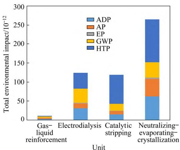
**Fig. 5** Total environmental impacts of gas-liquid vulcanization waste acid disposal technologies
