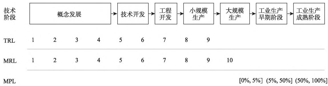
图1 技术开发的层次<sup>[18,19]</sup>Figure 1 Levels of technology development and mechanism<sup>[18,19]</sup>
