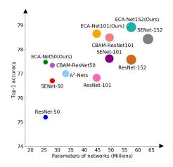
Figure 1. Comparison of various attention modules (i.e., SENet [14], CBAM [33],  $A^2$ -Nets [4] and ECA-Net) using ResNets [11] as backbone models in terms of classification accuracy, network parameters and FLOPs, indicated by radiuses of circles. Note that our ECA-Net obtains higher accuracy while having less model complexity.
