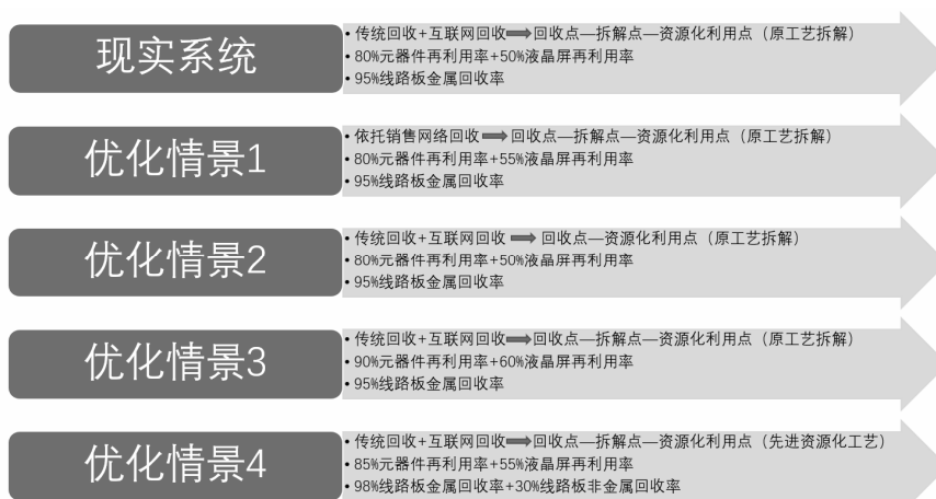
图2 废弃手机回收处理系统优化情景设置 Fig.2 Optimized scenario setting for discarded mobile phone recycling system
